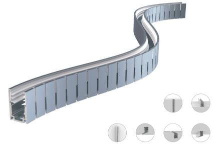
It is an expanded design of the serrated aluminum profile, and caters for the continuously streamlined aesthetics of curve shape. The secondary precision cutting process, not only maintains the advantage of clamping force, but also enables the two-way horizontal bending directions with super shape memory.
