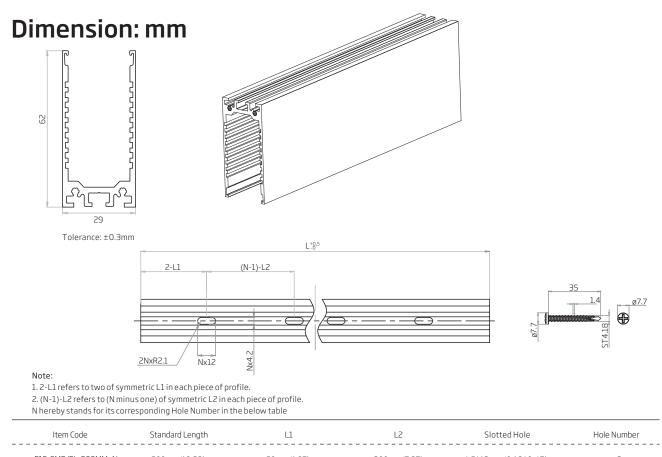
F15-SMR/PL-500MM-AL 50mm/1.97in 200mm/7.87in З 500mm/19.68in 4.5\*12mm/0.18\*0.47in F15-SMR/PL-1000MM-AL 1000mm/39.37in 100mm/3.94in 200mm/7.87in 4.5\*12mm/0.18\*0.47in 5 F15-SMR/PL-2000MM-AL 2000mm/78.74in 100mm/3.94in 200mm/7.87in 4.5\*12mm/0.18\*0.47in 10
